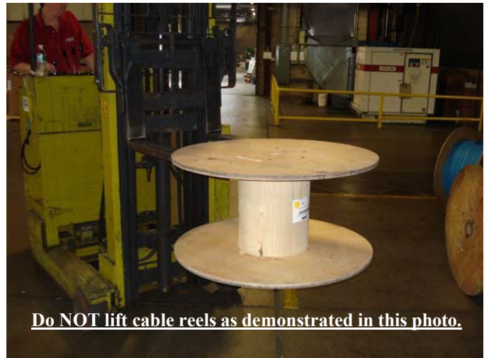
Never store cable reels on their side and never move cables reels in the manner shown above. (An empty reel was used for demonstration purposes)
