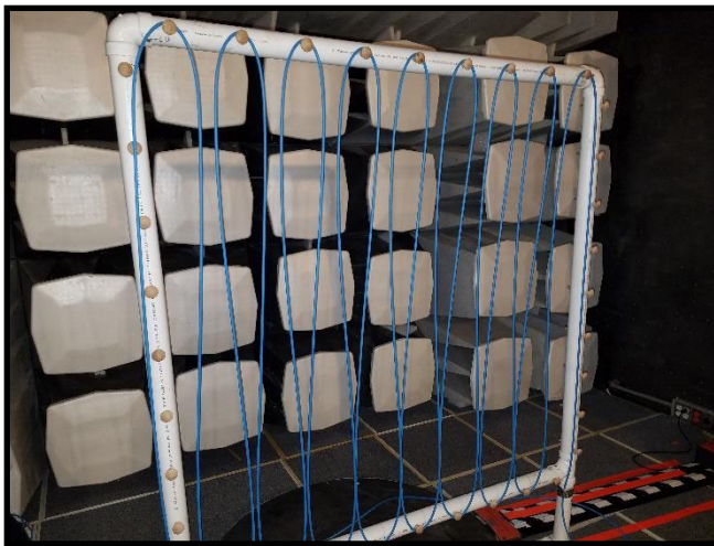
Figure 2. Cable arrangement within chamber
