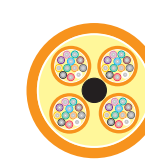
48-fibers (4 tubes of 12-fibers)
