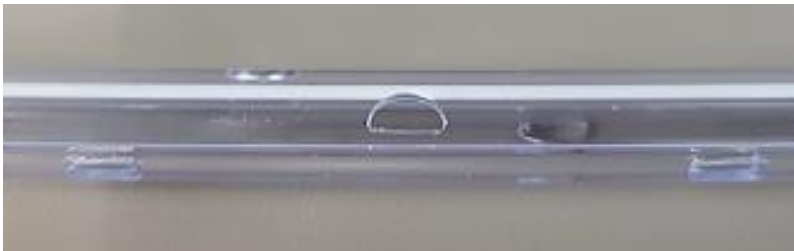
Nine .236”x.122” semi-circle punched holes spaced around the tube
