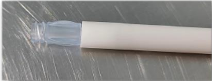
Pressfit luer into tube ID (no adhesive used)
