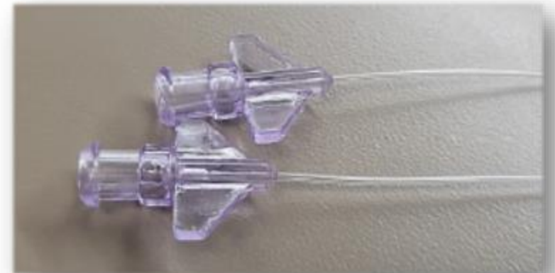
Luer and tube glued together with UV Adhesive, applied with syringe
