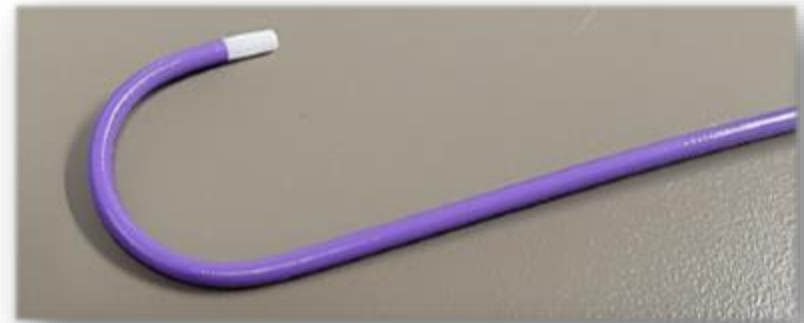
Braided tube formed into a hook using an annealing oven
