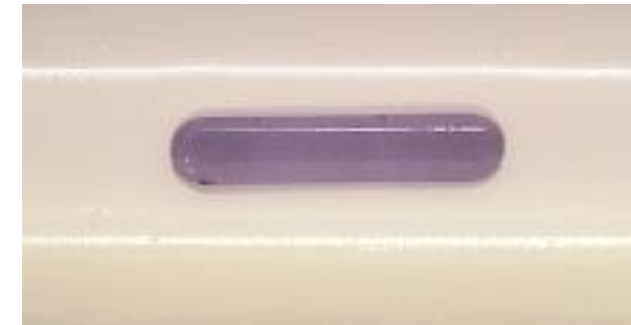
Thirteen .105”x.026” oval punched holes placed into specific lumens
