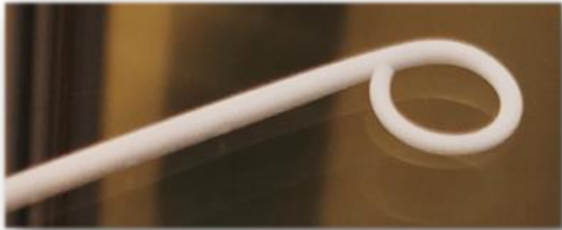
Tube Shaped with RF heating machine
