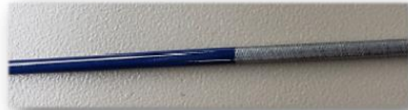
These two photos show one continuous tube. The core is nylon with metal braid covered with Pebax in varying durometers (7233, 6533, 5533, and 4533) to naturally give the tube different bend radii along the tube.
