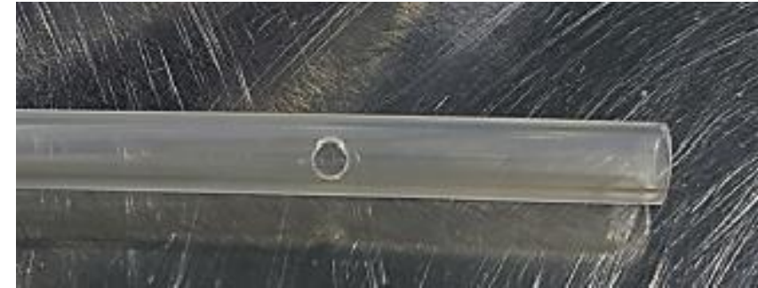
One Ø.118” drilled hole
