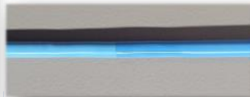
Vestamid Care ML94 and Pebax 4033 triple lumen tubes butt welded together
