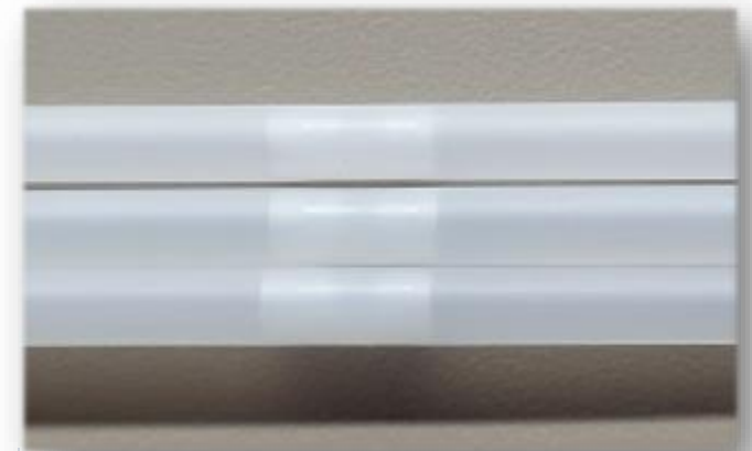
10mm long tube bonded inside longer tube
