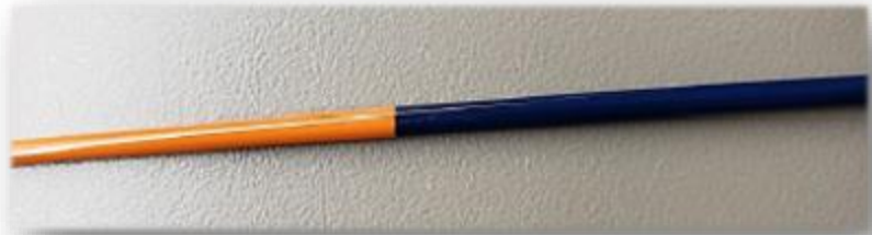
These two photos show one continuous tube. The core is nylon with metal braid covered with Pebax in varying durometers (7233, 6533, 5533, and 4533) to naturally give the tube different bend radii along the tube.
