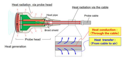
Figure 1 - Passive Thermal Heat Transfer
