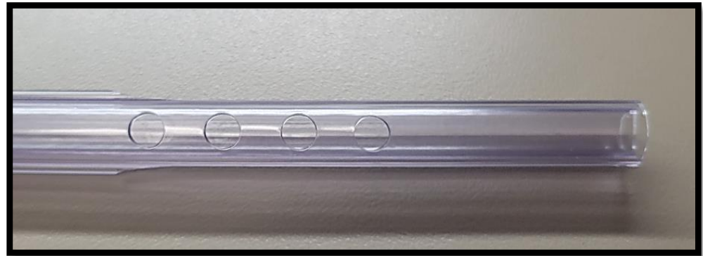
Two external lumens manually removed for the first 5 inches of the extrusion
