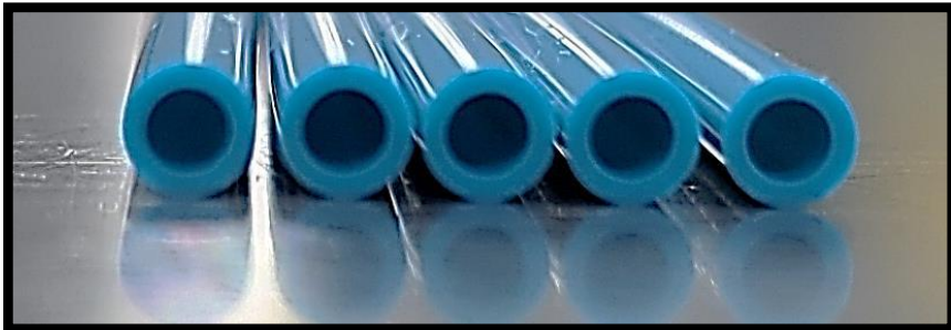
Trimmed on Cutting Block \text{Ø}.101'' to 63\text{cm} \pm .4\text{cm}
