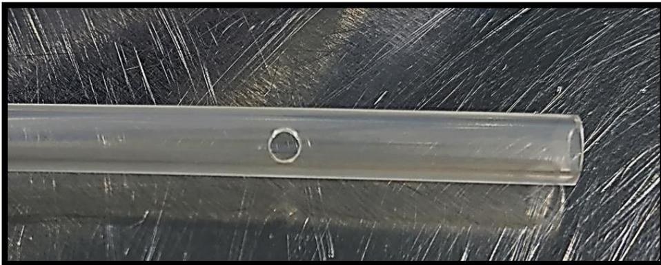
One  $\text{\O} .118$ " drilled hole
