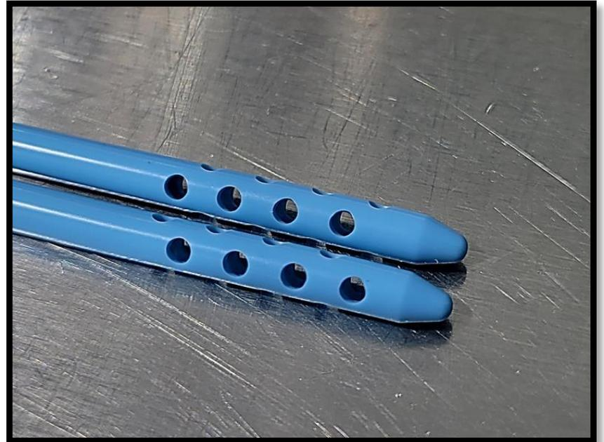
Sixteen  $\text{\O} .067$ " drilled holes spaced evenly around the tube
