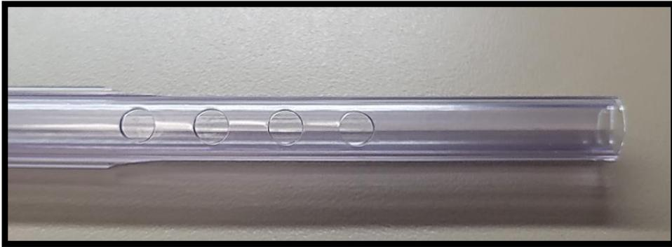
Four  $\text{\O} .20$ " drilled holes in a line
