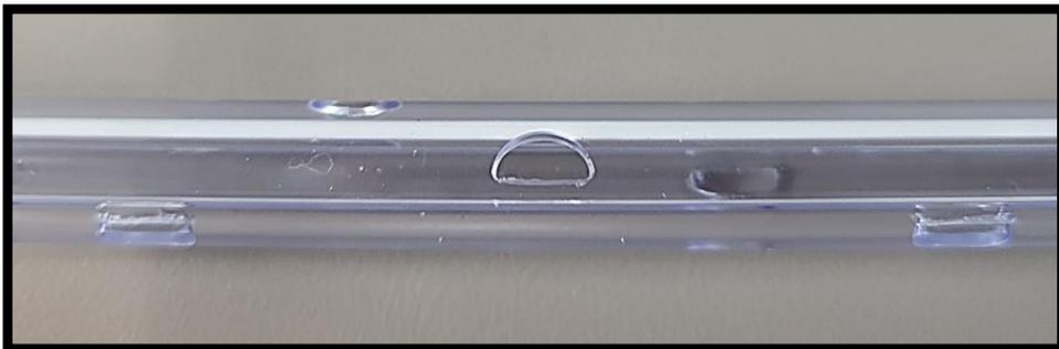
Nine  $.236$ "x $.122$ " semi-circle punched holes spaced around the tube
