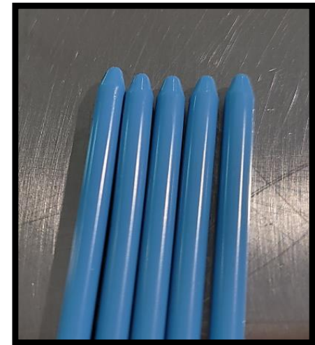
OD change from \text{\O} .130'' to closed tip with .039 radius over .118''
