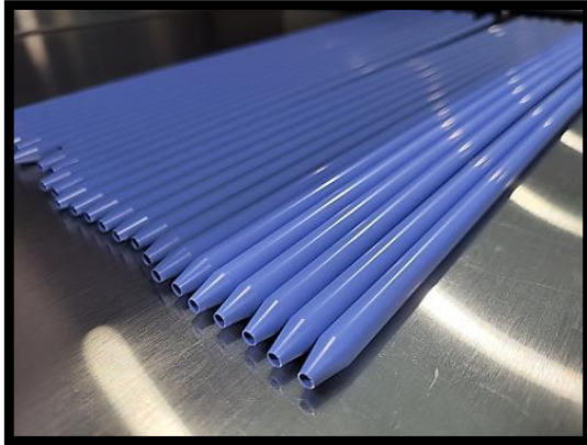
OD change from \text{\O} .341'' to \text{\O} .150'' over 0.385'' with consistent wall
