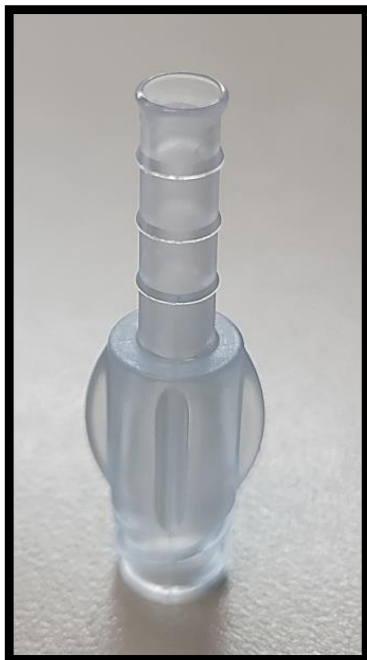
Luer with OD change from \text{Ø}.144'' to \text{Ø}.196'' over 0.065'' with consistent wall
