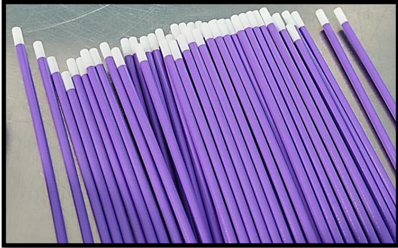
Braided purple Grillamid and Pebax 6333 tube butt welded to white Pebax 3533 tip
