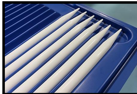
OD change from \text{\O} .356'' to \sim\text{\O} .050'' and ID change from \text{\O} .154'' to \text{\O} .040'' over 1.2''
