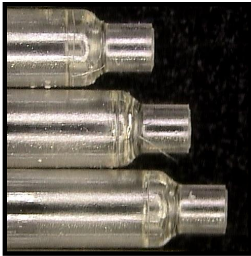
ID change from \text{\O} 1.58\text{mm} to \text{\O} .9\text{mm} over 1\text{mm} with consistent wall
